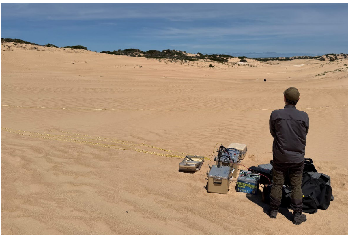
Figure 23. NMR sounding on the dune above Across Kartoo soak, October 2025. To complete a sounding, cables are laid out on the surface in a specific configuration.
