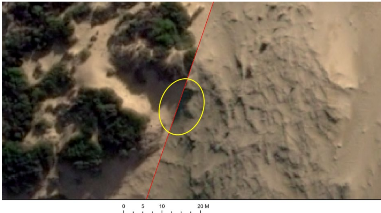
Figure 10. Enlarged view of the overlap / junction of two PN images, with the red line symbolizing the boundary of the junction area and illustrating the spatial mis-alignment (yellow ellipse). This view was established after removal of edge pixels by image masking.
