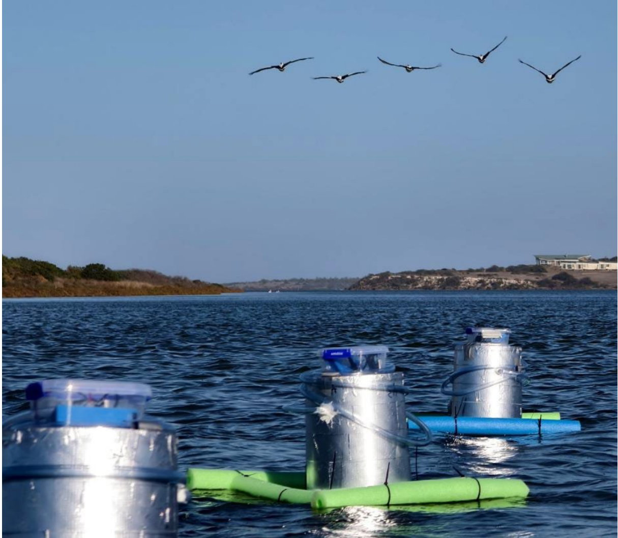
Figure 2. Floating chambers deployed and measuring CH 4 fluxes at Parnka Point, Coorong SA.
