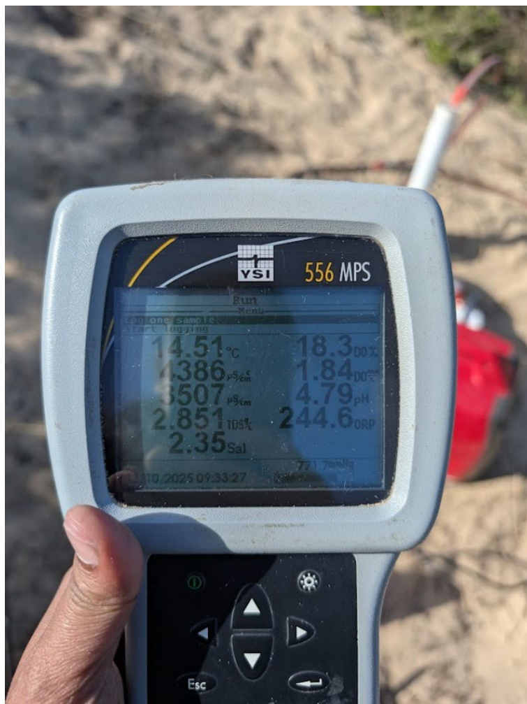
Figure 12. Example of water quality assessment using YSI 556 MPS multi-probe field meter (Photo credit: Sanjukta Das taken on 10 October 2025).
