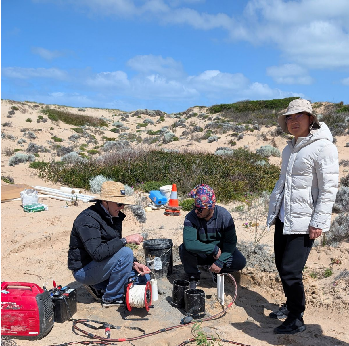
Figure 11. Use of the dip meter to measure watertable depth. The photograph shows Adrian Werner, Amin Gholami and Guohua Hou (left to right) (Photo credit: Sanjukta Das taken on 10 October 2025).
