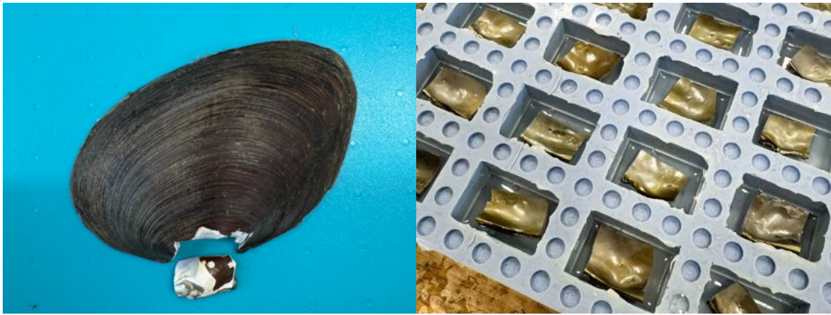
Figure 14. Section removed from umbo of a Lokeri (left) and umbos set in resin (right).
