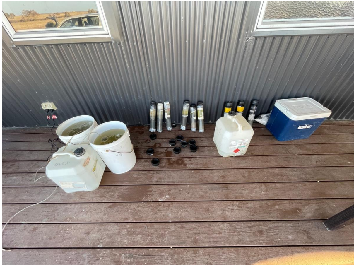
Figure A10: Setup for sulfide DGT processing. Deployed DGT probes can be seen on the left with site water being circulated over them.
