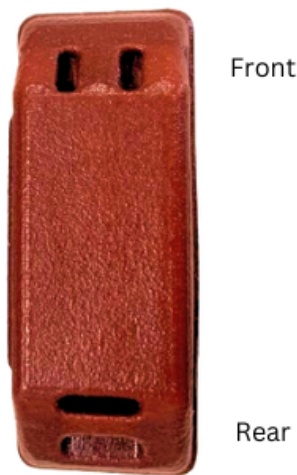
Figure 4: Image of the base of the GPS unit with the front and rear labels corresponding to the orientation of the unit on the duck
