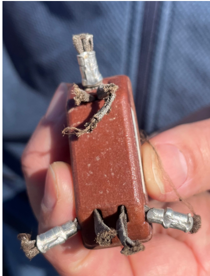
Figure 16: PP11F GPS unit as it was found in the Coorong. The broken Teflon was separated from the rest of the harness, and the crimps are still intact as they were when it was deployed.
